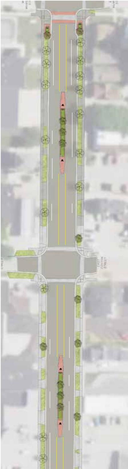
The Continuous Two-Way Turn Lane is wide enough to accommodate a median in certain areas where the distance from a major intersection meets the required 150 foot clearance distance for designated DOT connecting highways. No planted medians would be allowed in these spaces allotted for left-hand turns. In some areas, parking and street trees would run along the outer street edge and provide a better sense of scale by closing the visual gap across the wider street.
