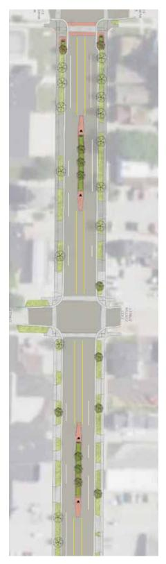
The Continuous Two-Way Turn Lane is wide enough to accommodate a median in certain areas where the distance from a major intersection meets the required 150 foot clearance distance for designated DOT connecting highways. No planted medians would be allowed in these spaces allotted for left-hand turns. In some areas, parking and street trees would run along the outer street edge and provide a better sense of scale by closing the visual gap across the wider street.
