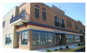
This example shows the use of a recessed entry to identify its location, and changes in material and wall plane to break up the side facade.
