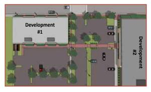
This illustration shows two developments on adjoining lots sharing parking and an access drive. A sidewalk connects the two developments through the parking area.
