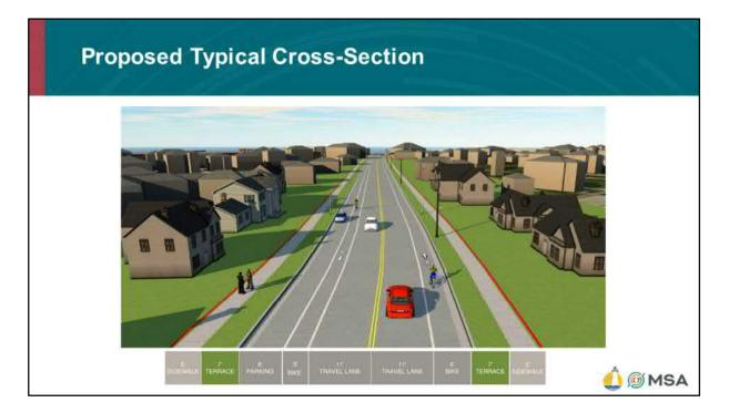
Here is a display showing the proposed cross-section dimensions for the majority of the project length. The total curb to curb width will be 41 feet, generally, with parking on the west side of the street only. There will be bicycle width accommodation between the curbs, as shown here. The sidewalks will generally be 5 feet wide compared to 4.5 feet wide existing.
