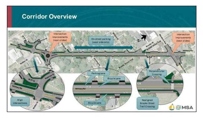
This exhibit shows the proposed roadway overlaid onto an aerial photograph of the area. On the left, south end, the Superior Street intersection will be adjusted so it comes into Military Road at a 90 degree angle and will line up with Walker Street, for safety. Note on the exhibit that the west-side, on-street parking will extend between Grove Street and Brooke Street. At Brooke Street, the multi-use trail will be re-aligned so it crosses 90 degrees to the street, for safety.
