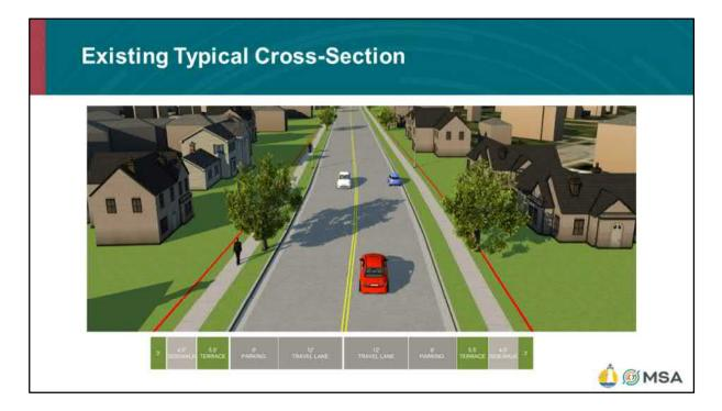
To give an idea of how the proposed work compares with the existing conditions, here is a display showing the existing cross-section dimensions for the majority of the project length. The total curb to curb width is currently 40 feet, generally, with parking on each side of the street. There are currently no bicycle accommodations in the street cross-section.
