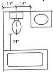
A water closet or urinal may not be located closer than 15 inches from its center to any side wall, partition, vanity, or other obstruction, nor closer than 30 inches center to center, between water closets or urinals. There shall be at least 24 inches clearance in front of a water closet to any wall, fixture, or door.
