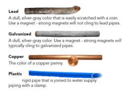
Water service material has changed over time. The four main materials are lead, galvanized or iron pipe, copper, and polyethylene or plastic. Lead was initially used because it's stable and malleable. Plumbers found it easy to work with. As a matter of fact the word "plumbing" is derived from the Latin word for lead, "plumbum" and dates back to the Roman era.
